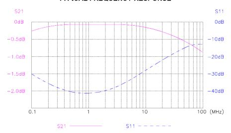
The MI 1005 is characterized by Return Losses of more than -10db at frequencies of 100 MHz and a low insertion loss of less than -1,1 dB.
